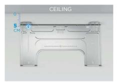
**STEP 2**: Move down the plate until the punch hole to the **SPOT A**
